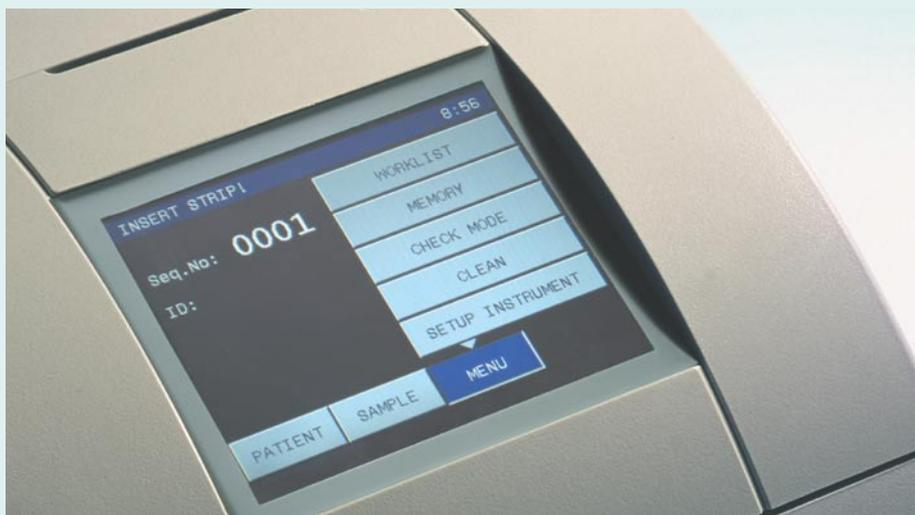
Like the preceding model, the innovated LAURA® reader proves to be based on the principle of reflection photometry and it allows for use of seven and ten-parameter diagnostic strips (HeptaPHAN® LAURA and Dekaphan® LAURA) which are **completely automatically recognized** by the reader. In comparison with the ori-
