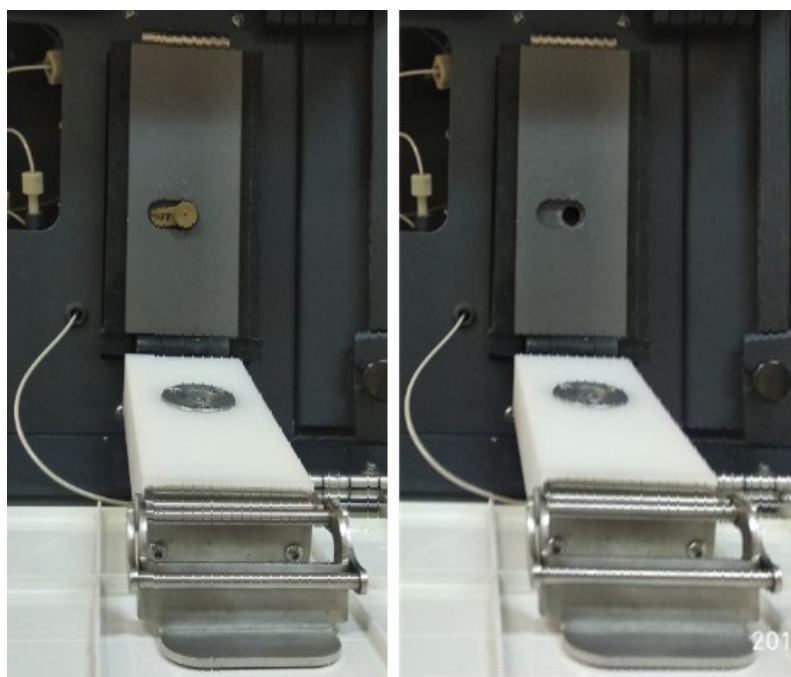
Figure 8: Close up views of the open column holder (with and without column)
