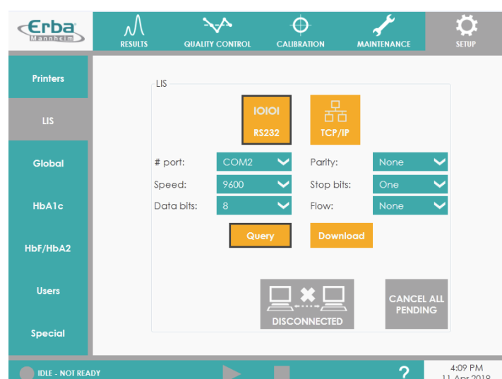
Figure 24: LIS Connection for Serial (RS232) mode
